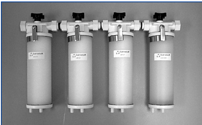
SolmeteX, Inc.'s Amalgam Effluent Management System for treating flows from large dental facilities.
