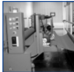
Needle punched non-woven textile emerging from the loom and rolling onto the bolt.
