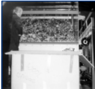
Loading the "card" with recycled polyester fleece fiber and wool.
